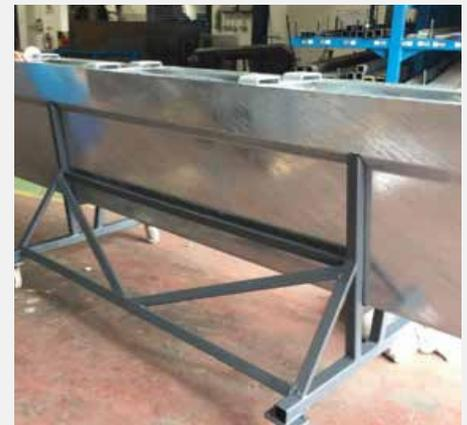
A “mobile wheeled assembly frame” that allows a safely restrained barrier to have its wheels fitted anywhere rather than being limited to a work area bench, was introduced to ensure that consistency and quality is maintained between manufactured units.
